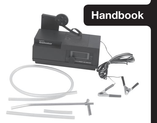
Gastester is an exhaust gas analyser that works on the "hot wire" or "thermal conductivity" principle: the thermal conductivity of exhaust gas varies in proportion to the amount of carbon monoxide present. Exhaust gas is pumped through the Gastester by an externally mounted pulse pump.
